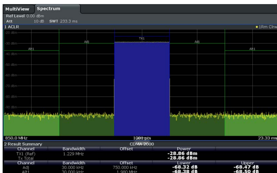
Fig. 4-2: Measuring the channel power and adjacent channel power ratio for CDMA2000 signals with zero span (Fast ACLR)
